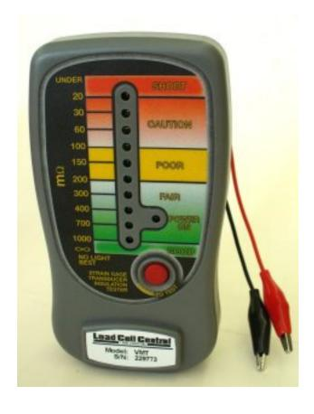
LOAD CELL/SENSOR INSULATION TESTER
