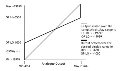
Method of Calculating **Output Low** & **Output High** from known output values
