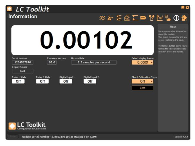
**Relay 1 State** – Indicates whether relay 1 is on or off.
