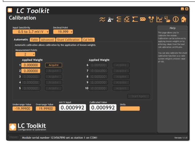
**Measurement Points** – Enter between 2 and 10 measurement points. These are the points at which weights will be applied. This process will linearise as it calibrates.
