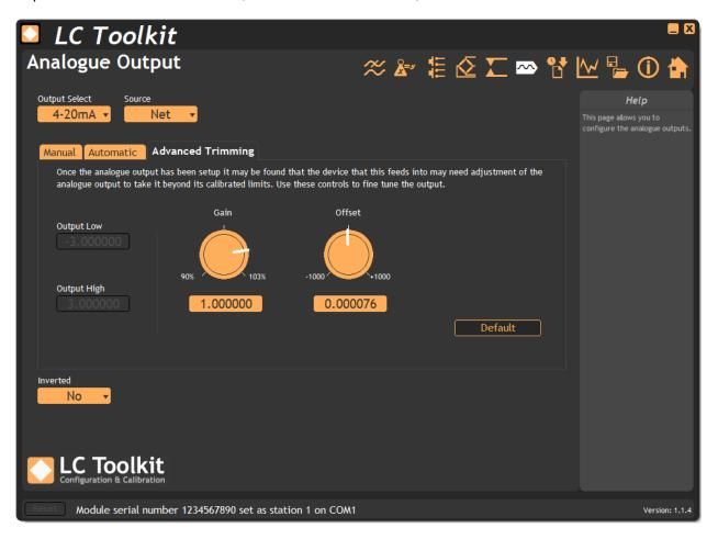
**Gain** – Alter the analog output gain by clicking and dragging the pointer on the virtual knob.
