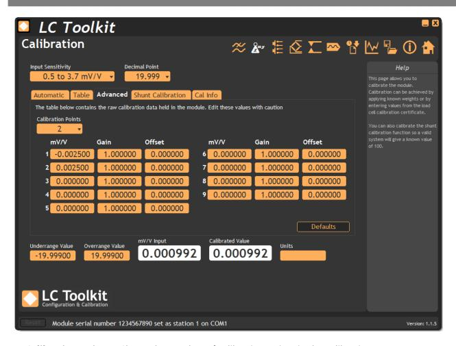
**Calibration Points** – Shows the number of calibration points in the calibration.
