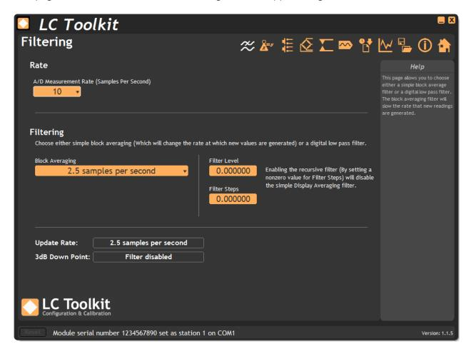
**Rate** – Here the basic selection of A/D measurement rate can be selected. The slower rate will have an improved noise free resolution.
