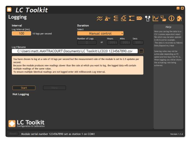
Once the logging starts the actual achieved log rate will be displayed at the bottom of the window. This is useful for diagnostics such as when a heavily burdened PC is slowing the log rate.
