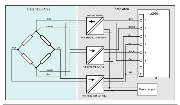
Because the barriers are fully isolated, the **REF** connection **MUST** be made to ensure that the LCD20 input stage is biased correctly.
