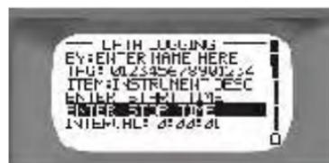
**Interval:** Use set value keys to set logging intervals H:MM:SS from 01 second to 9H:59M:59Sec
