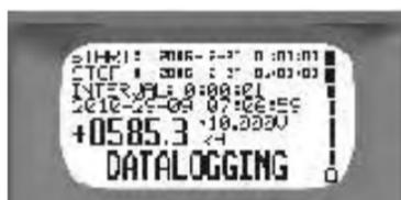
*For instant datalogging whilst in the LC Display mode, insert the SD card and press enter to start and enter to stop.*
