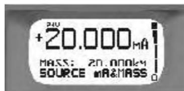
Use value set keys to change mA value then press enter to output new value (+ Steady)
