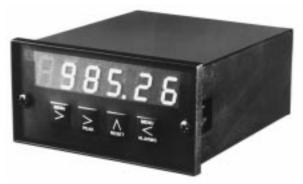
The VPI is a low cost solution to a wide range of monitoring and control applications. By simple front panel push button setup, one meter with a universal signal conditioner can be programmed to display DC or AC voltage or current, any of 6 popular thermocouple types, 100 Ohm platinum RTD's, strain gauges and process signals. All at the price of a single function meter!
