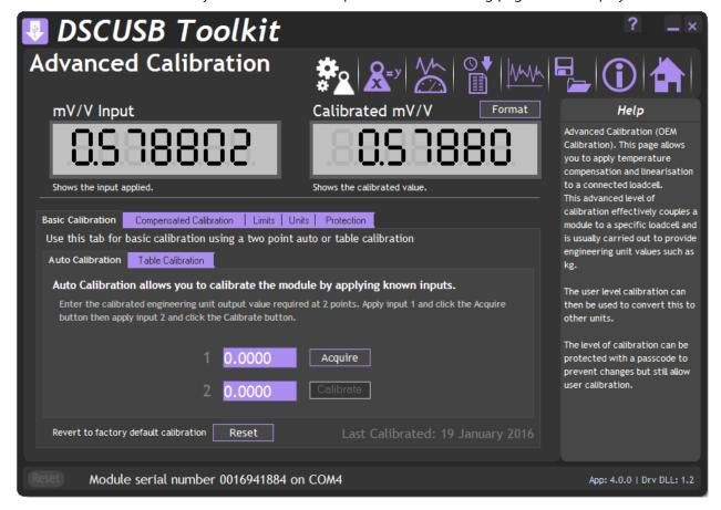
This page allows you to calibrate the module using various methods, set limits, perform system zero and set units description.
