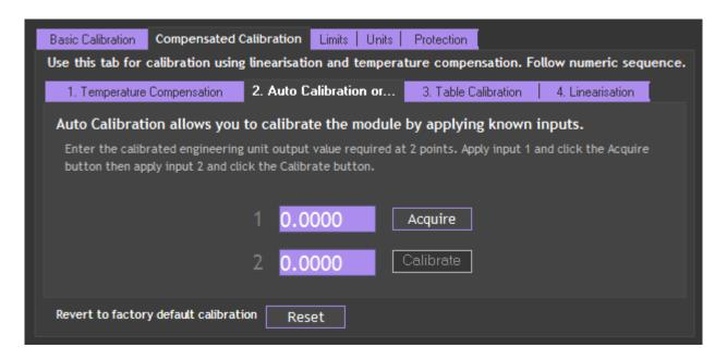
The automatic calibration requires that you apply two known (ascending) weights in sequence. Just enter the required engineering unit value for the two weights in the fields marked 1 and 2.
