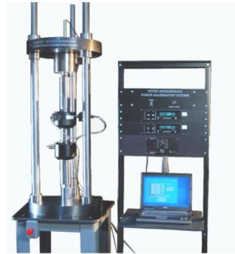
This is an example of a typical calibration press.
